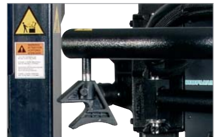
Gentle demounting with the bead depressor
