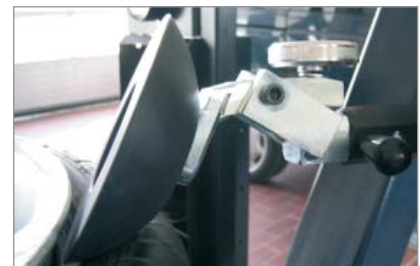
The plastic bead breaker disc is a useful accessory to prevent any damage to the rim
