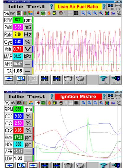
The Suite package includes the Coda Ignition Analysis System. This tool allows you to quickly identify faults within the ignition system and combined with the high speed scope software will allow labscoping of any of the sensors. Testing of coils and modules to a pass/fail status is also an integral part of the unit.
